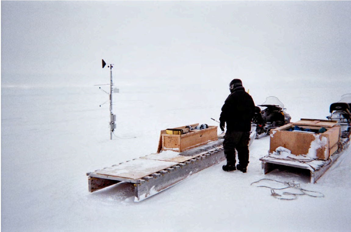
The data collection site near Sanikiluaq, with one of the community monitors. The weather station transmits data by radio to a receiver in the community.
