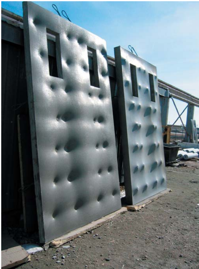
Figure 4a. The concrete panel on the left (foreground) is cast directly from the fabric formwork rig shown in Fig. 1. The Panel to its right was cast using this first panel as a mold.
