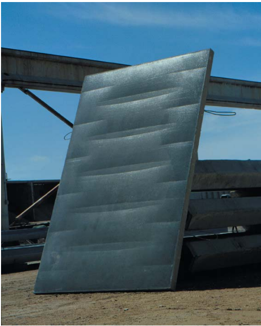
Figure 11. Fabric-cast mold for the Figure 12 GFRC shell panel. This mold was produced from the Figure 10 intermediate support design.
