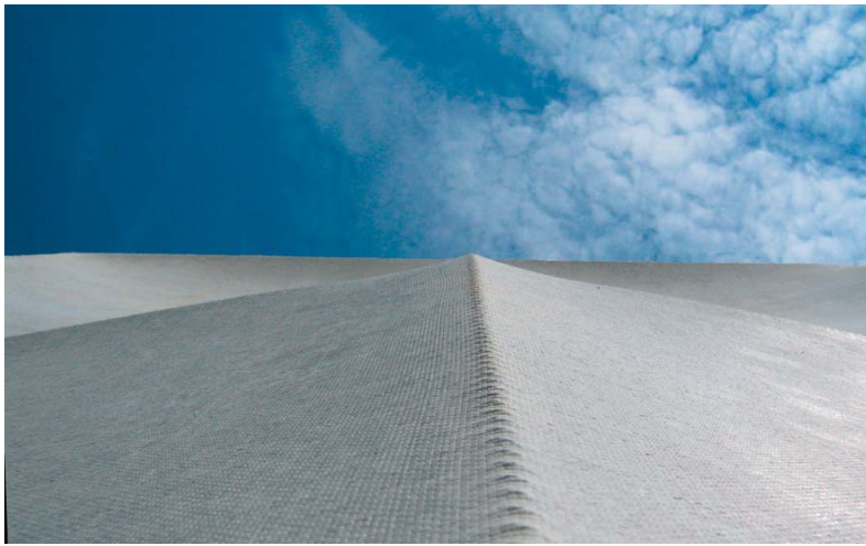
Figure 15. The "inverted cast" shell panel shown in Figure 9 (left) and cast from the direct-cast panel shown in Figure 8.
