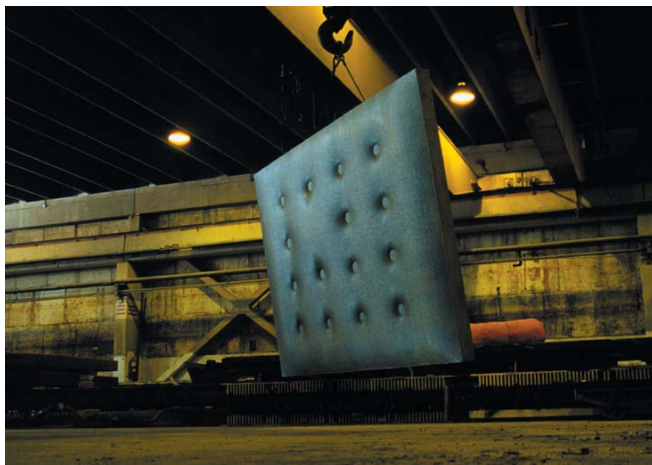
Figure 5. Another "direct-cast" concrete panel produced from the same fabric formwork membrane illustrated in Fig. 2. In this case, however, intermediate supports were provided in a grid pattern.
