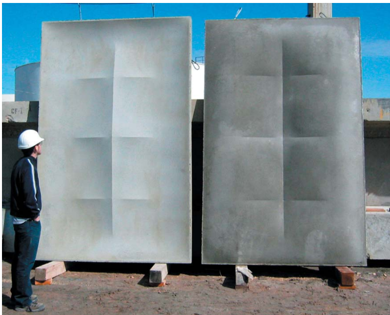
Figure 9. The Shell Panel on the left was cast from the “direct-cast” panel on the right (the same direct cast panel shown in figure 8).
