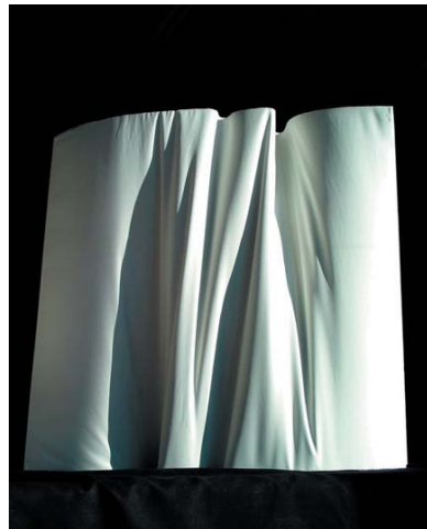
Figure 20. Spray plaster model of a thin-shell spray concrete panel.
