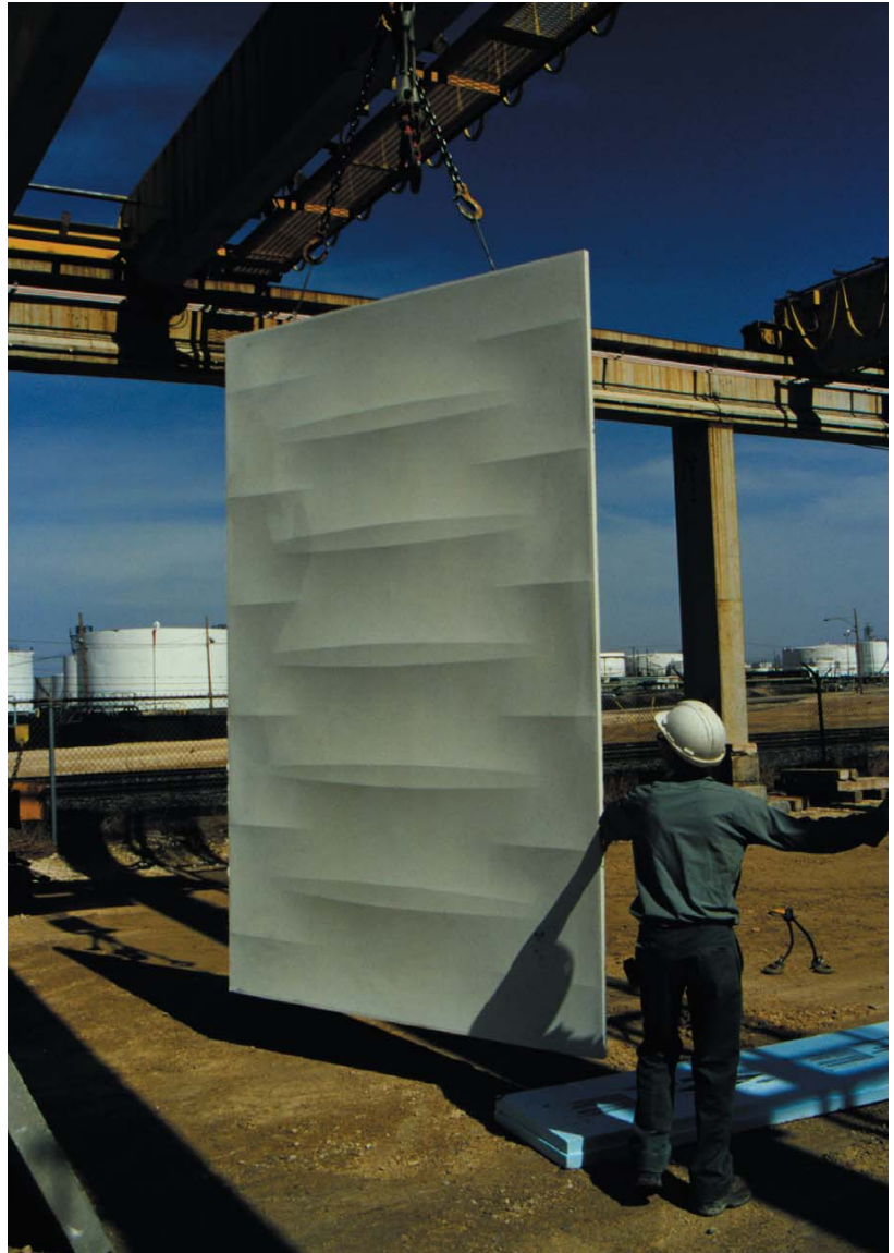
Figure 12. Lightweight GFRC shell panel produced from the Fig. 10 "direct-cast" mold. This panel varies in thickness from 13 mm (0.5 in. ) to ( 38 mm (1.5 in.)).
