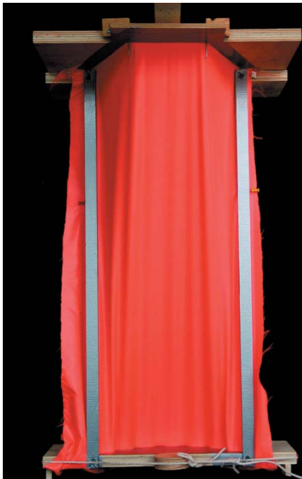
Figure 18a. Model fabric formwork pre-stressed in a "cradle" rig.
