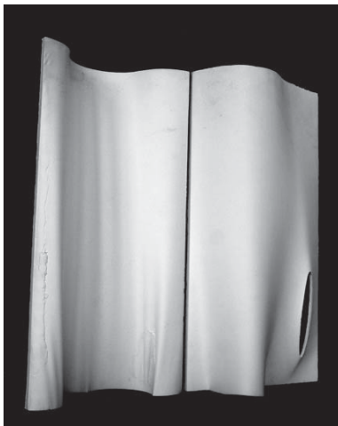
Figure 19. Spray plaster model of thin-shell spray concrete panels.
