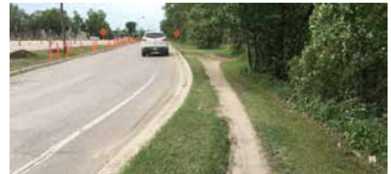
Figure 17: Examples of a gap in the network where a desire line marks the preferred location for a pathway.
