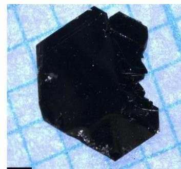
**Figure 2:** CVT grown crystal of  $\text{MoS}_2$
