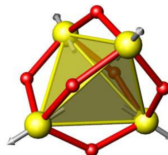
Figure 2: Tetrahedral spin arrangement on metals (yellow) with oxide (red) bridges.
