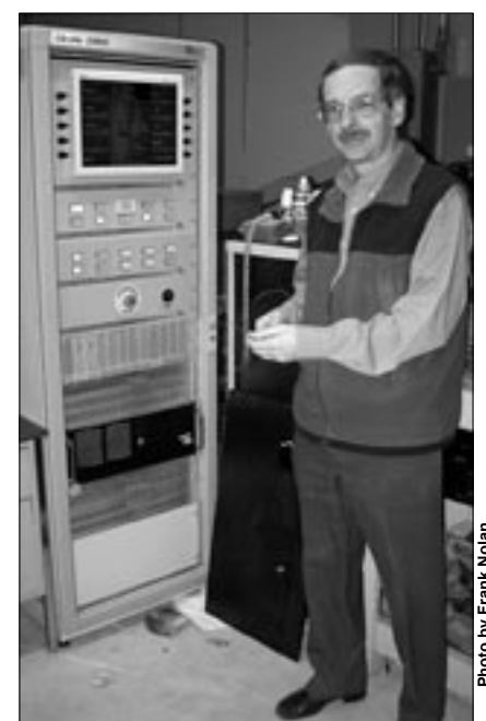
Norman Richards, mechanical and manufacturing engineering, and the Gleeble Thermal Simulator, which measures the performance of repaired superalloys under extreme temperature conditions.
