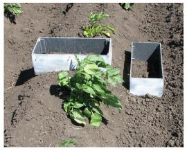
Chambers for measuring N losses as nitrous oxide (N<sub>2</sub>O) emissions from soil in irrigated potatoes, Carberry, MB (photo: S. Parsonage)
