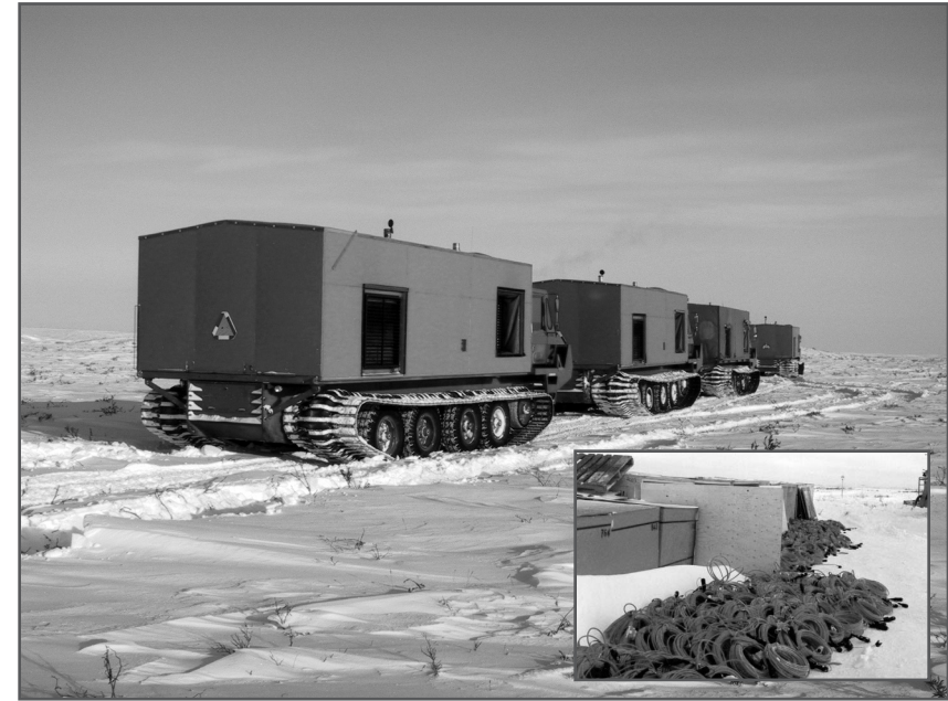
Seismic operations in the Mackenzie Delta, winter 2002. Near Tuktoyaktuk, NT. Vibrator Energy Source and Recording Equipment. Photo by Pete Millman, Devon Canada Corporation.
