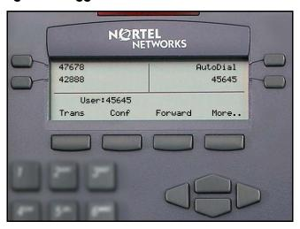
Figure 6: Logged on to an IP Phone 2002 using an IP Phone 2004
