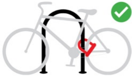
U-Lock secures rear wheel and frame.
