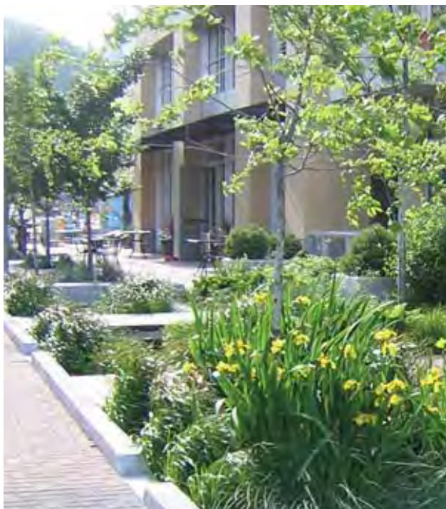
Rain gardens stormwater management
