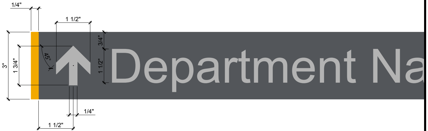
WF 1.1 - Line Panel Detail
