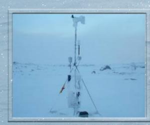
Icing problems, S1 at elevation 721 m
