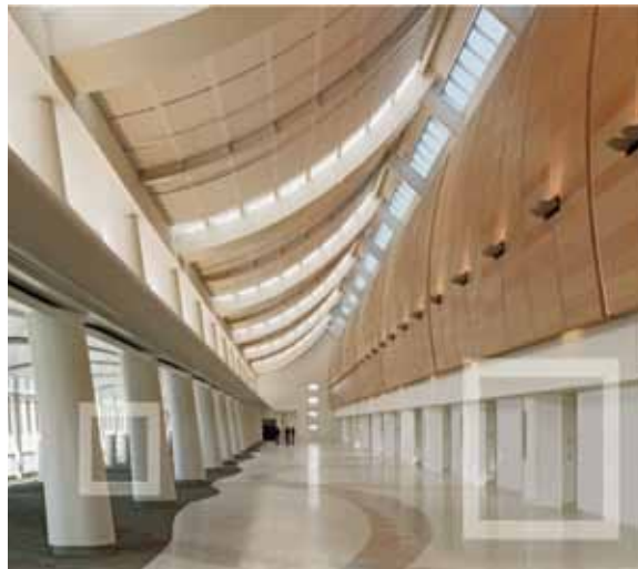
SJ Airport: Displacement ventilation is integrated into the wall and terminals at Mineta San Jose International Airport (Architect: Gensler)
