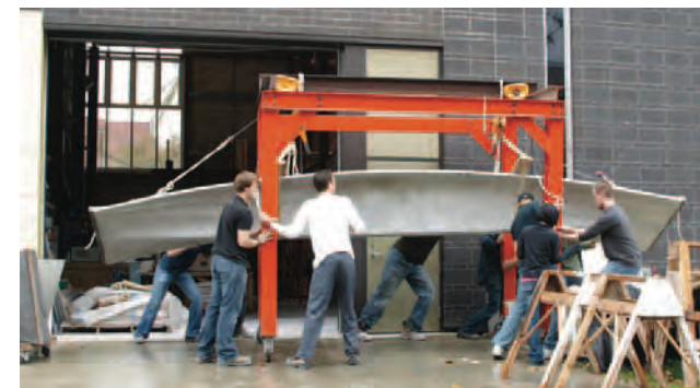
The first thin-shell structural vault produced from a fabric-formed mold.
