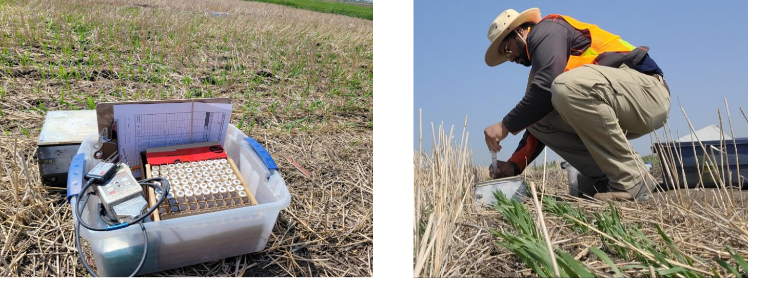
Figure 2 and 3. Example of field equipment used for extracting N 2 O on the field composed of field sheets, evacuated vials, syringes and static vented gas chambers
