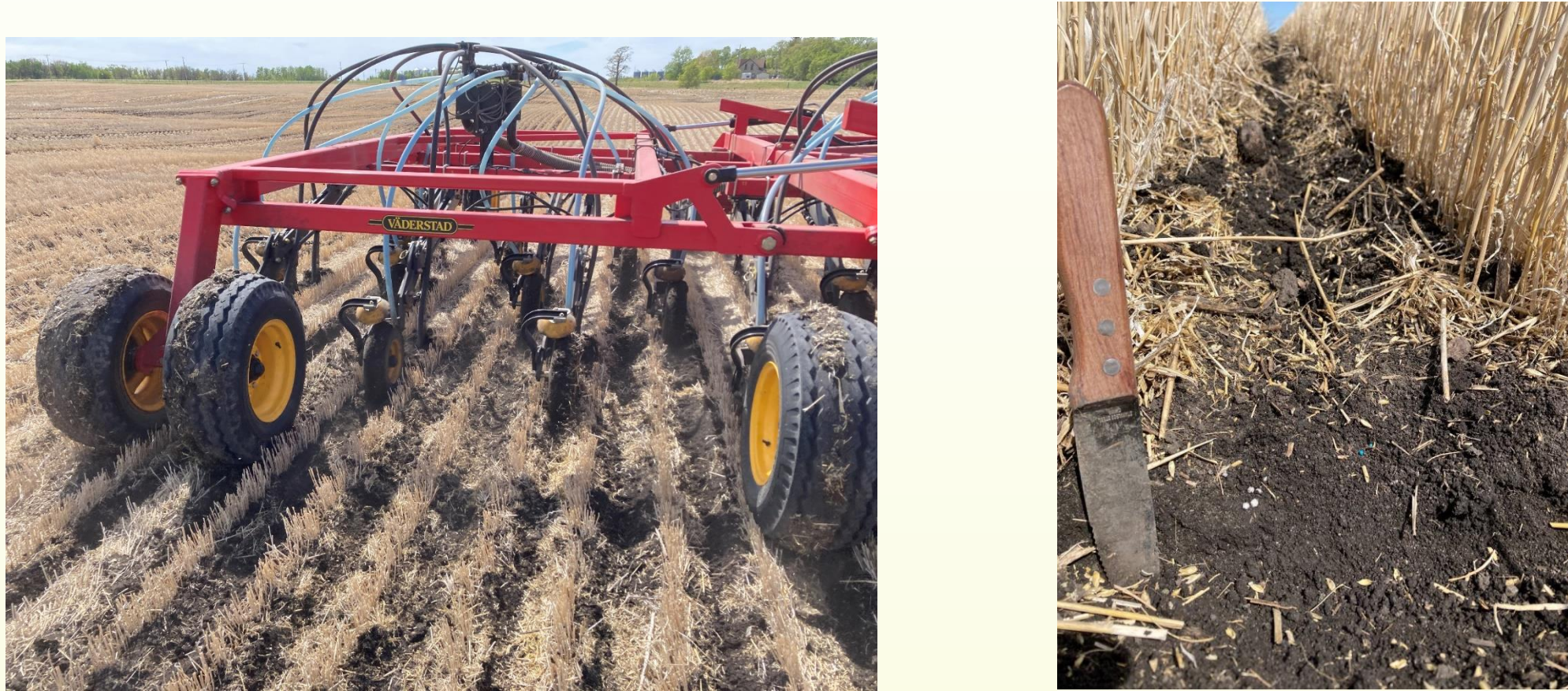
Figures 5,6. Seeding and sideband fertilization (left). Note fertilizer placement to the side and below the canola seed (right).
