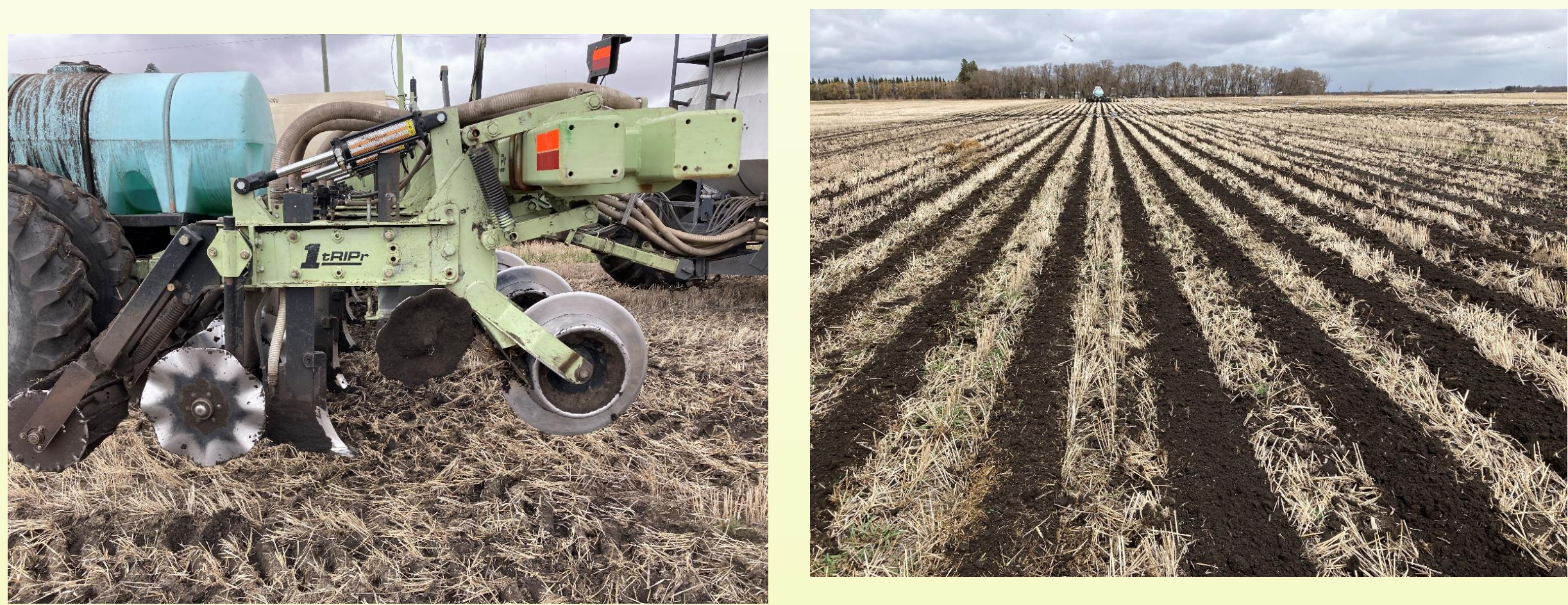
Figure 1-2. Strip till application of nutrients prior to seeding in 10" wide bands on 30" row spacing.
