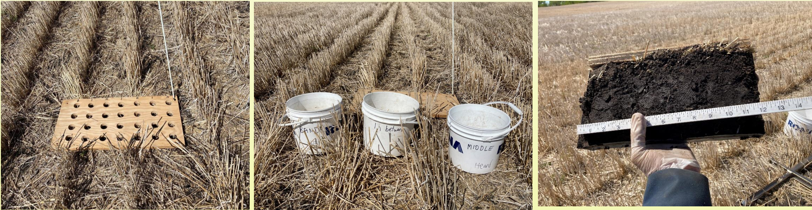
Figures 7-9. Soil sampling template (left), 3 pails (middle) and cross-section sample (right).
