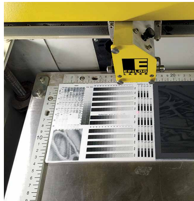
A laser marking test on porcelain tile, for Grace Nickel's Espalier tile series. Instead of firing in a kiln, ceramic material is sintered onto porcelain by a laser cutter.
