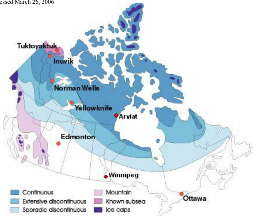
Figure 8: Extent of Permafrost Coverage in Canada
