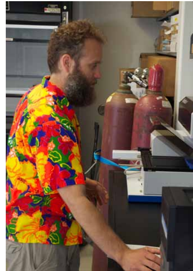
Pictured Right: The Nellie Cournoyea Arctic Research Facility also houses cutting edge analytical equipment. Shown here is Dr. Jessie Carrie using a mercury analyzer. This is a new innovative instrument that saves significant time. It can produce measures of elements such as mercury in minutes rather than days and in sample sizes as small as a single copepod. Photo Credit: Jason Jorgenson.
