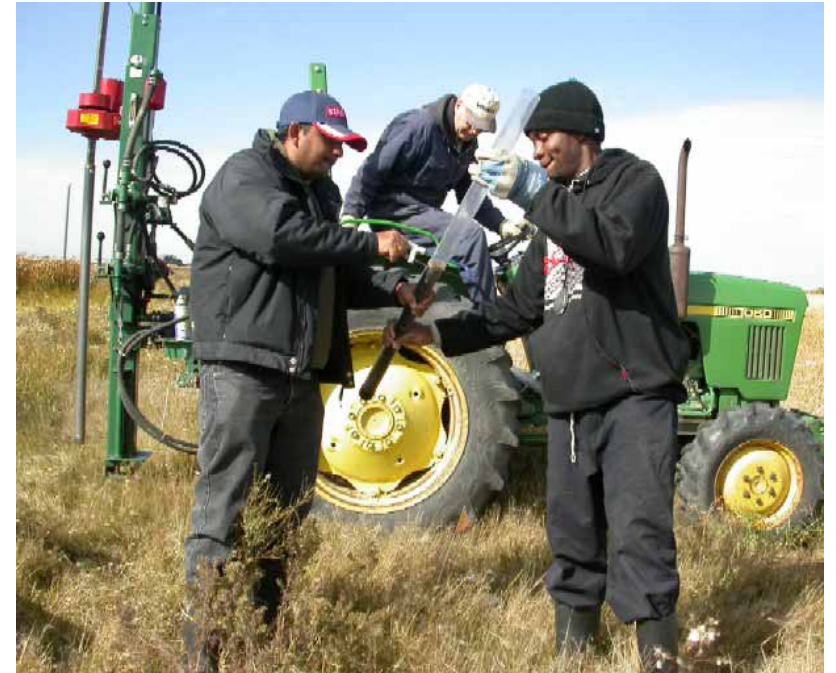
Deji and Nandakumar Cutting a Core MZTRA Soil Cores Segmented for Determination of Nitrous Oxide Production and Consumption MZTRA
