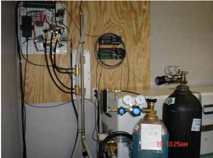
Sampling Manifold from the NCLE Plots
