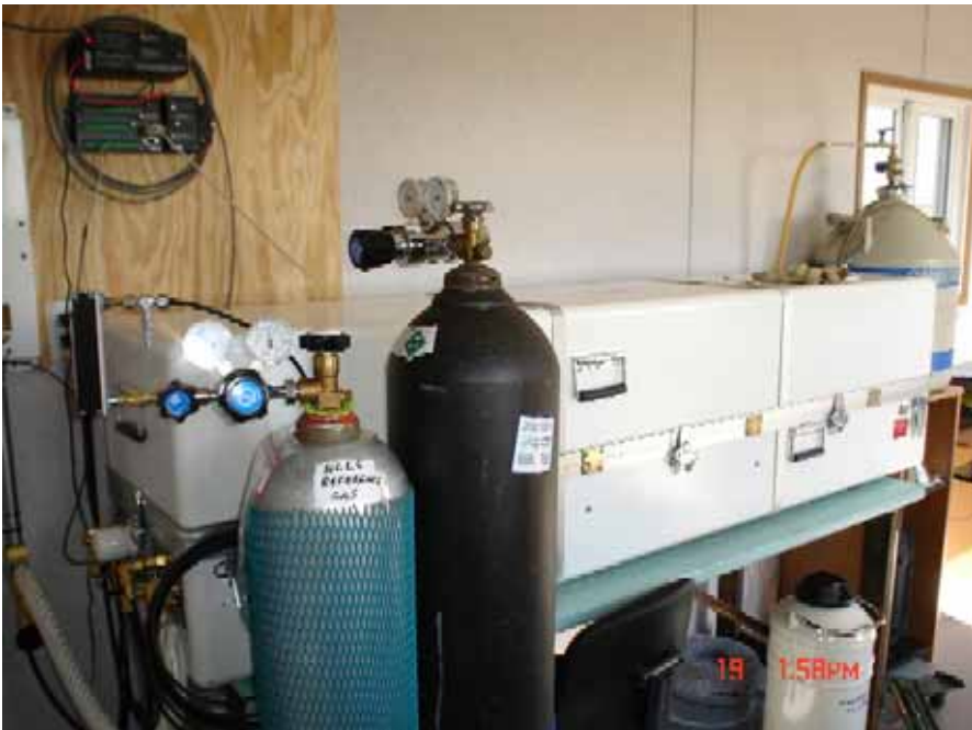
NCLE Tunable Diode Laser for N_2O and CO_2 Field Fluxes
