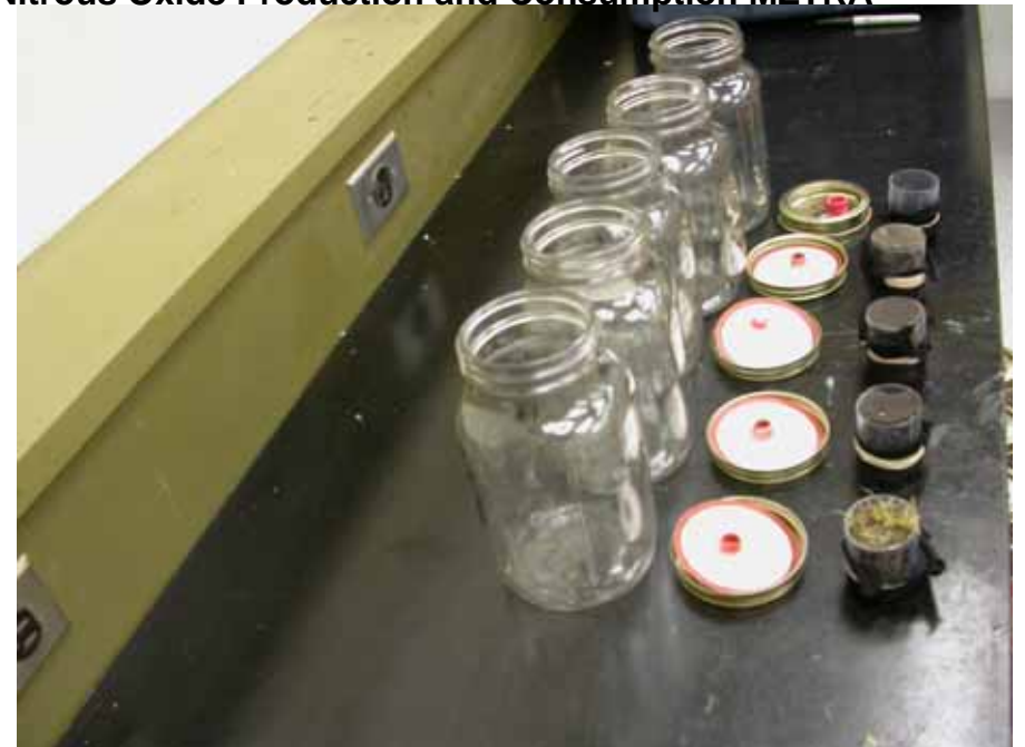
Deji and Nandakumar Cutting a Core MZTRA Soil Cores Segmented for Determination of Nitrous Oxide Production and Consumption MZTRA
