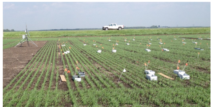
Figure 3. N source test plots growing spring wheat at Warren, MB with chambers for measuring N 2 O-N losses (photo: K. Baron)
