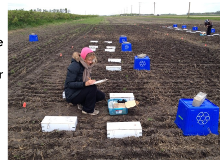
Figure 4. Measuring N 2 O-N losses from N source test plots at Glenlea, MB in fall following application of anhydrous ammonia (photo: K. Baron)
