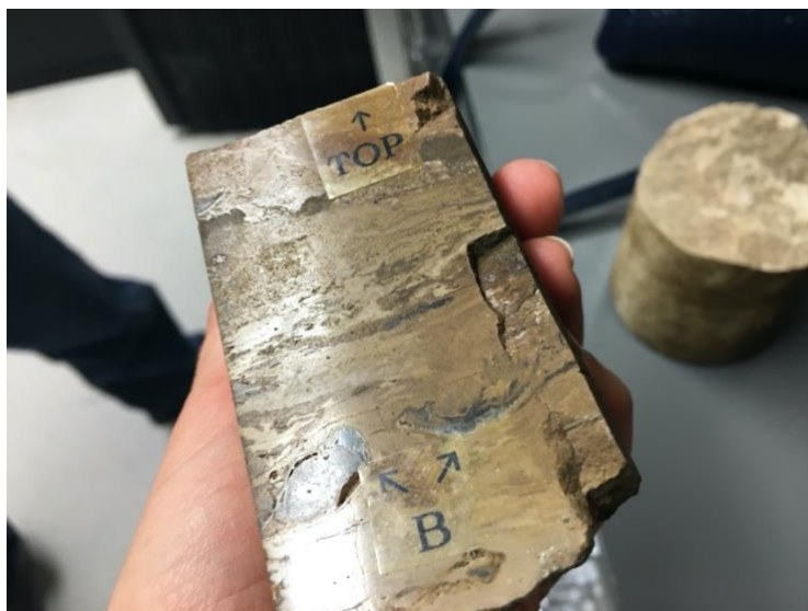
Figure 7: Piece of core with oil traces
