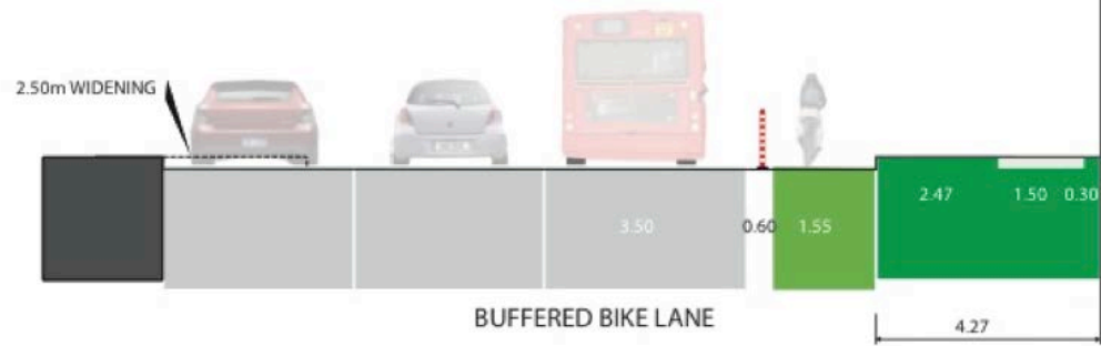
Figure 4: Chosen design for buffered bike lanes (City of Winnipeg, 2012)
