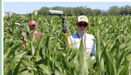
Figure 1. Corn reflectance being measured by the GreenSeeker® (back) and the CropCircle™ (front).
