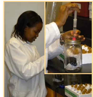
Waraidzo Chiyoka samples for N 2 O from soil mixed with digested cattle manure. Waraidzo is a graduate student with Dr. Zvomuya.
