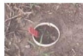
Figure 1. Root exclusion cylinder consisting of a PVC pipe inserted to a 10' depth from which plants were removed to isolate the PRS™ from plant root competition.
