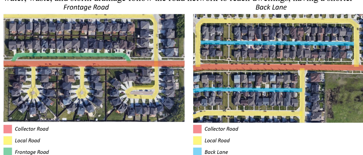
Figure 9 - Frontage roads and back lanes used along collector roads in Bridgwater Forest.
